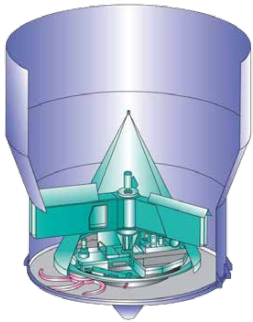
ROTARY DISCHARGE MACHINE
